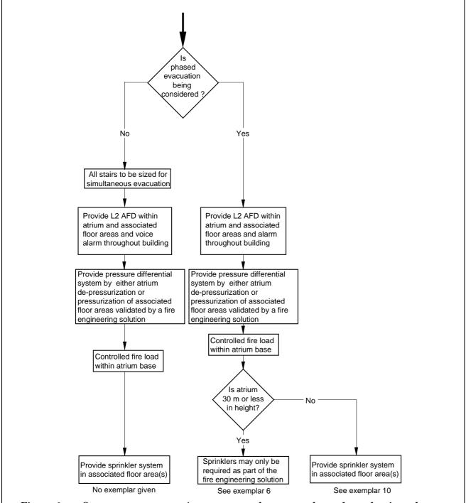
Figure 3e — Occupancy category A: occupants who are awake and, predominantly, are familiar with the building — Atrium enclosed with fire-resisting construction and using pressurization
