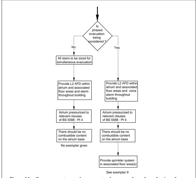
Figure 3d — Occupancy category A: occupants who are awake and, predominantly, are familiar with the building — Atrium enclosed with fire-resisting construction and using pressurization
