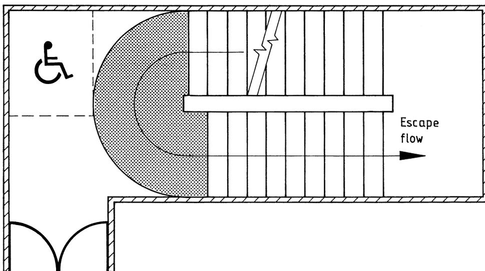
b) Provision where access to the wheelchair space is counter to the access flow within the stairway
