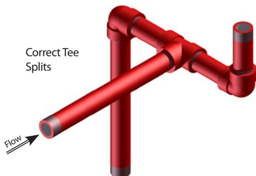
Figure 43 - Bull tee orientation "correct"
