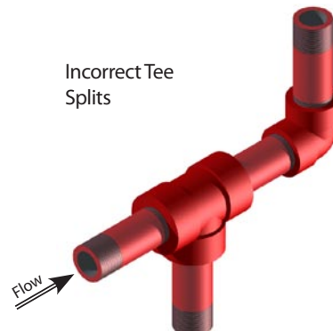
Figure 44 - Bull tee orientation "incorrect"
