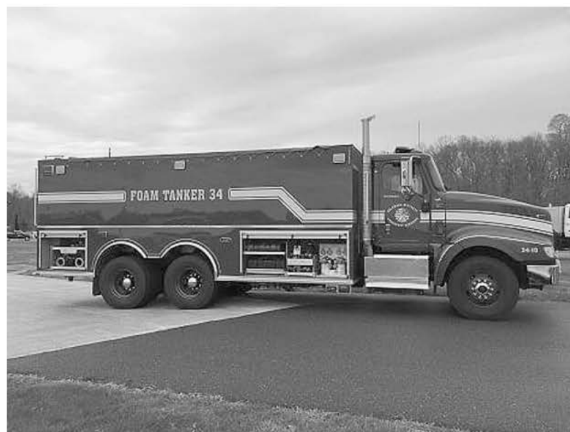
FIGURE A.3.3.5.1 Foam Tanker.
