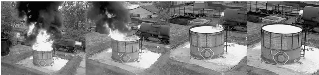
FIGURE H.3.2(c) Extinguishing Sequence, FFF, Subsurface Injection.
