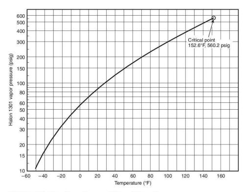
FIGURE C.2.1.1(a) Vapor Pressure of Halon 1301 vs. Temperature.
