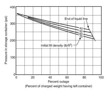
FIGURE H.1(c) Calculated Pressure Recession for 360 psi Storage.
