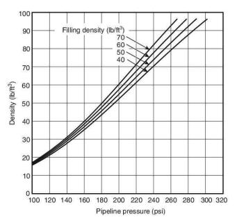
FIGURE H.1(g) Pipeline Density for 360 psi Systems Based on Constant Enthalpy Expansion.
