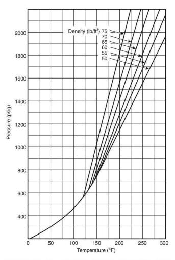
FIGURE E.1.1(c)  $\,$  Isometric Diagram. Halon 1301 Pressurized to 360 psig at 70  $^{\circ}\text{F}.$
