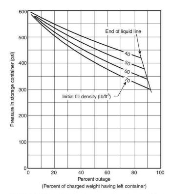
FIGURE H.1(b) Calculated Pressure Recession for  $600~\mathrm{psi}$  Storage.
