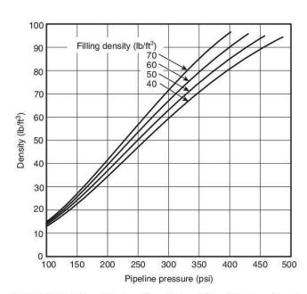
FIGURE H.1(f) Pipeline Density for 600 psi Systems Based on Constant Enthalpy Expansion.
