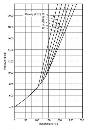
FIGURE E.1.1(e)  $\,$  Isometric Diagram. Halon 1301 Pressurized to 600 psig at  $70\,^{\circ}\text{F}.$
