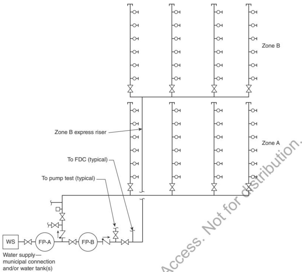
FIGURE A.10.5.2(n) Zones Up to the Level of Fire Department Pumping Capacity Using Pumps in Series — Two Vertical Standpipe System Zones Example.
