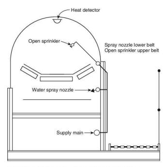
FIGURE A.7.2.3.3.1(b) Typical Hooded Conveyor.
