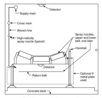
FIGURE A.7.2.3.3.1(a) Typical Conveyor Belt Protection.
