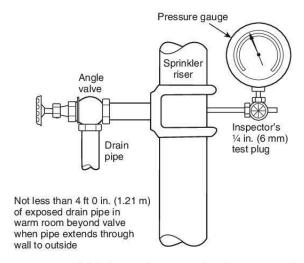
FIGURE A.6.3.3.6 Drain Connection for System Riser.
