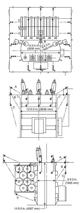
FIGURE A.7.4.4.1 Typical Transformer Layout.
