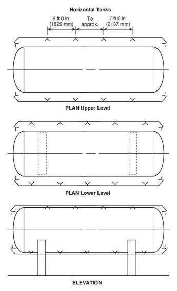
FIGURE A.7.4.2.3 Typical Horizontal Tank Protection.
