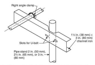
Note: Pipe stand brackets are now replacing the old style pipe stand without the bracket. The bracket makes installation easier and allows for adjustment horizontally and vertically. The standard bracket is made to fit 2 in. (50 mm), 2½ in. (65 mm), or 3 in. (80 mm) pipe stands.
