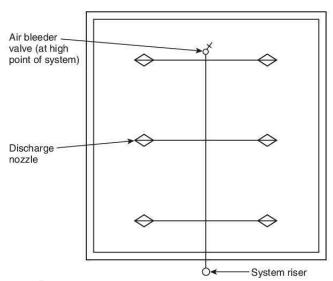
Note:  $\Phi$ - High-speed water spray nozzle in the pendant position.
