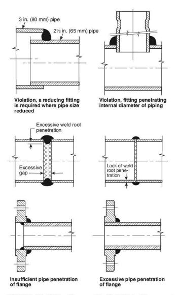
FIGURE A.5.5.2(b) Unacceptable Weld Joints. [For correct pipe penetration of flange, see Figure A.5.5.2(a).]
