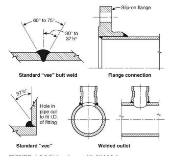
FIGURE A.5.5.2(a) Acceptable Weld Joints.
