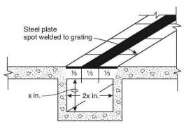
Drainage trench with steel plate and grating cover
