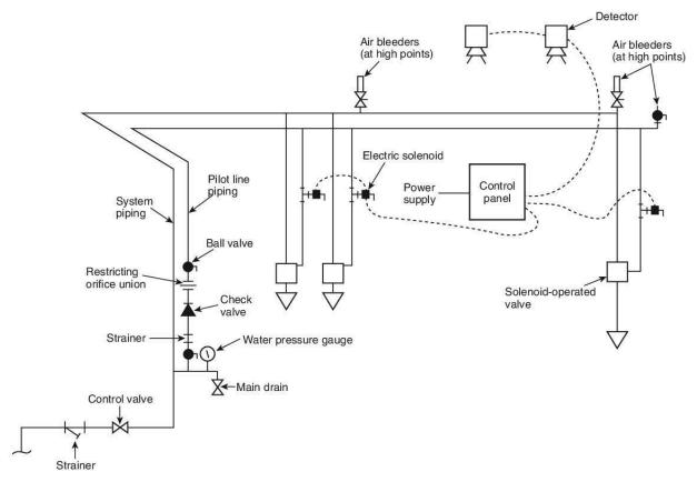
FIGURE A.12.3.10(b) Ultra-High-Speed System Using Solenoid-Operated Valves.
