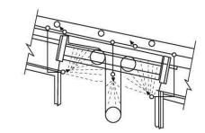
Elevation of typical take-up roller protection
