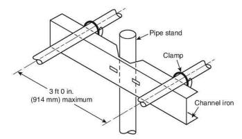
$\label{eq:figure_figure} \textbf{FIGURE} \ \ \textbf{A.6.3.2.2.8(d)} \quad \ \ \textbf{Multiple Pipes Supported by One Pipe Stand.}$
