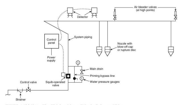
FIGURE A.12.3.10(a) Ultra-High-Speed System Using Squib-Operated Valve.
