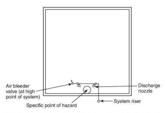
FIGURE A.12.3.1.1 Ultra-High-Speed Local Application for a Point of Hazard.
